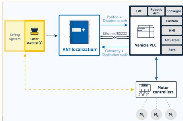
ANT localization<sup>+</sup> estimates a vehicle's distance from the desired virtual line (offset). It then communicates this data directly to the PLC, as well as providing virtual tags and a recommended speed.
