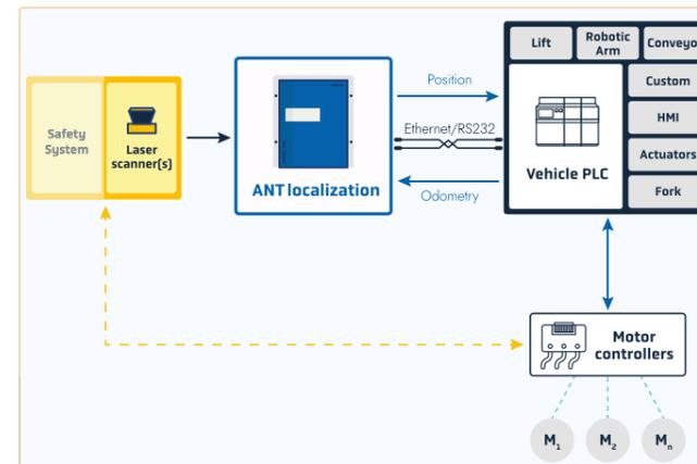
ANT localization provides a vehicle's coordinates directly to the PLC.
