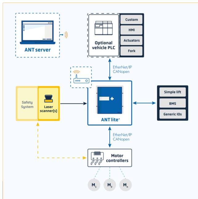
ANT lite+ provides commands directly to a vehicle's motor controller or via the vehicle's PLC (e.g. to interface with specific devices).
